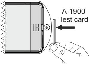
**Manual TEST with the A-1900 Test card (not included).** This card is available only after request. In order to test the device, you must place the card on the side of the indications. This operation lasts as long as the card is present.
