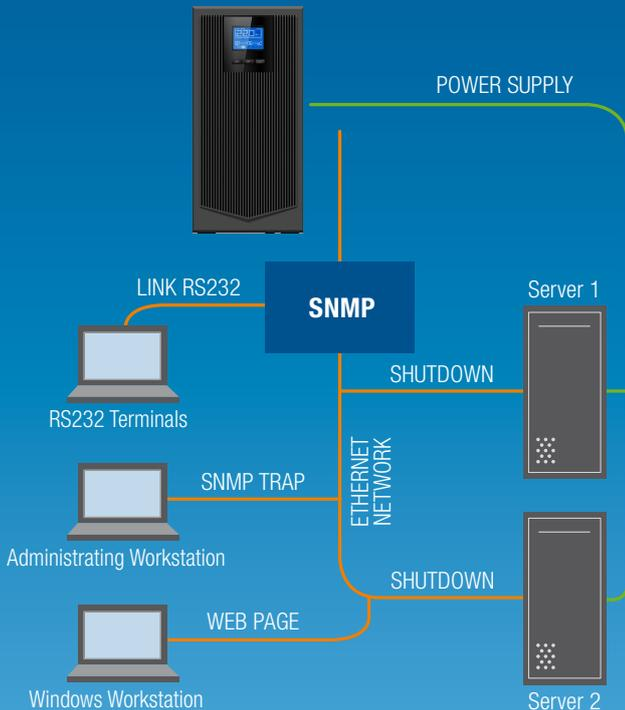
UPSilon 2000 CD is packed with UPS. it has the function of remote monitor and control UPS through LAN.
