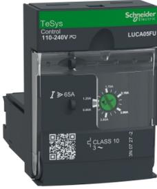
Standard control unit, TeSys Ultra, 3P, 1.25 to 5A, 690VAC, thermal magnetic protection, class 10, 110 to 240VAC/DC coil
