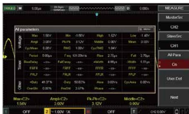
● Automatic Measurement of Waveform Parameters
