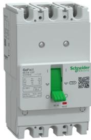
Circuit breaker, GoPact MCCB 125, 3 poles, 10kA at 415VAC, 63A rating, TMD trip unit, fixed thermal protection
