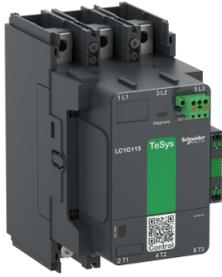
High power contactor, TeSys Giga, 3 pole (3NO), AC-3  $\leq 440\text{V } 150\text{A}$ , standard version, 100...250V wide band AC/DC coil
