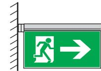
Flag mounted installation on a wall using the special mounting bracket contained in the package.
